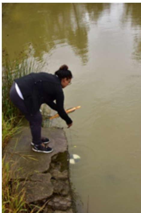
Anji uses an inexpensive Secchi disk to determine water clarity, while Nick uses an expensive multi-parameter probe (Aqua Troll 500) to measure water chemistry in McKenzie Creek.
