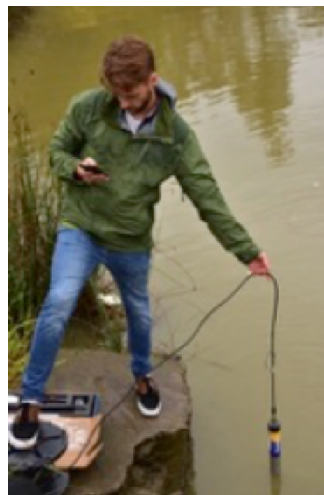
Anji uses an inexpensive Secchi disk to determine water clarity, while Nick uses an expensive multi-parameter probe (Aqua Troll 500) to measure water chemistry in McKenzie Creek.
